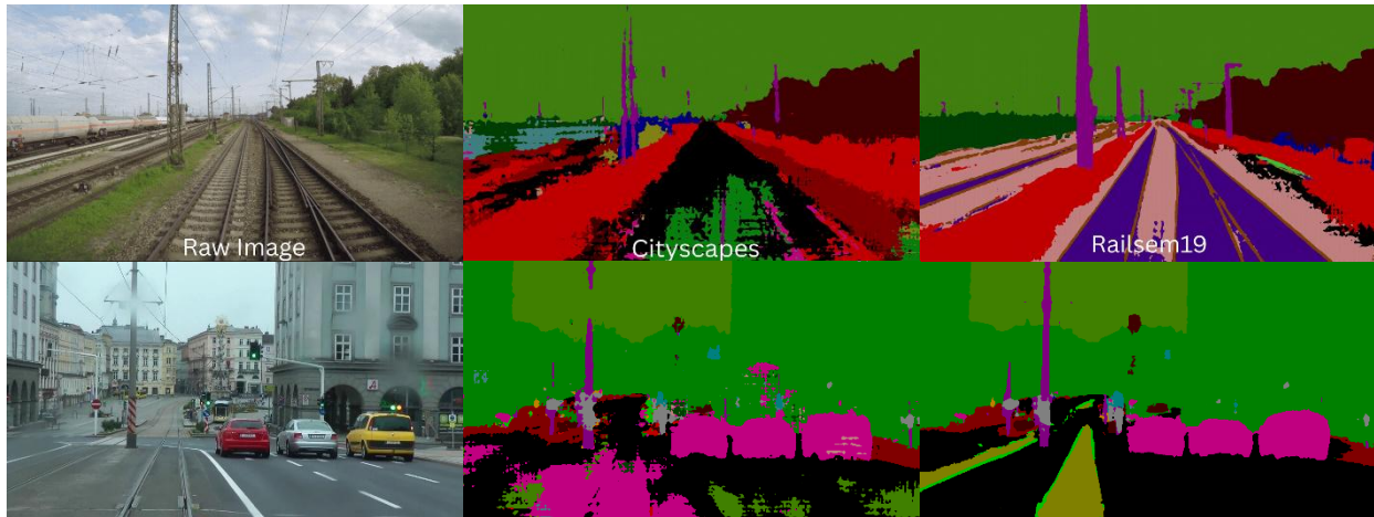
Figure 3: Example BiSeNetV1 segmentation results. Left: raw image. Middle: Cityscapes model. Right: Railsem19 model.
